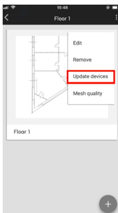
OTA (over-the-air) firmware updates allow you to upgrade the firmware on your lighting devices using the HubSense® Commissioning mobile app. The firmware update is automatic (the new firmware is stored and downloaded from the cloud). To update external firmware (not related to Bluetooth® mesh), the user must have a firmware file (in a zip format) and upload it to the HubSense® Commissioning mobile app.
