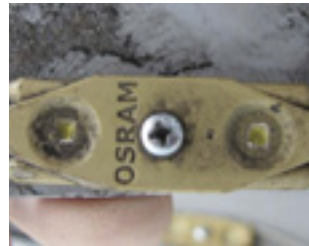
Dirt on top of the LED surfaces
